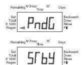
In Alternator Systems when a unit is waiting to initiate the first cycle step of regeneration, "REGEN PndG" is displayed.
