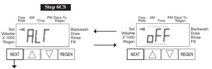
Step 6CS – This display will not appear if  $1.0 \Gamma$  was selected in Step 2CS. Allows selection of one of the following using  $\blacktriangle$  or  $\blacktriangledown$ :
