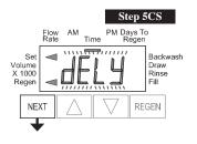
Step 5CS – Press ▲ or ▼ to select to regenerate immediately on 0 or at delayed time. Immediately on 0 can only be selected if Volume (gallons) was selected in step 4CS and a meter must be installed. Delay is the only option for the other Step 4CS selections. Press NEXT to go to Step 6CS. Press REGEN to return to previous step.
