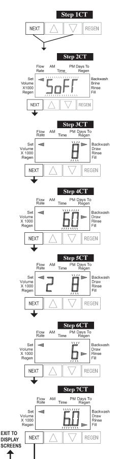
**Step 1CT** - Press NEXT and  $\nabla$  simultaneously for 5 seconds and release. If screen in Step 2CT does not appear, the lock on the valve is activated. To unlock press  $\nabla$ , NEXT, REGEN,  $\triangle$  in sequence, then press NEXT and  $\nabla$  simultaneously for 5 seconds and release.
