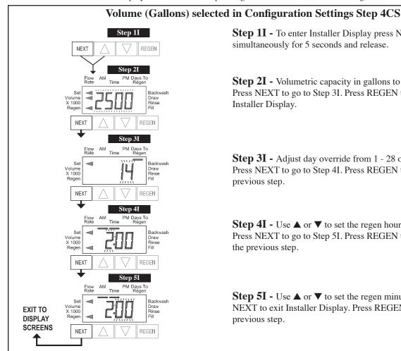
**Step 1I** - To enter Installer Display press NEXT and ▲ simultaneously for 5 seconds and release.
